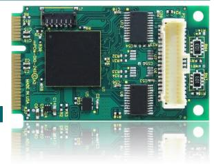
The mPCIe-DIO-24S is a type F1 PCI Express Mini Card (mPCIe) and optional cable assembly (DSub 37-pin Male connector) designed to be easily panel-mounted in any application environment. It uses the high speed PCI Express bus to transfer digital data to and from the card. The digital I/O is compatible with 8255 PPI chips making it
